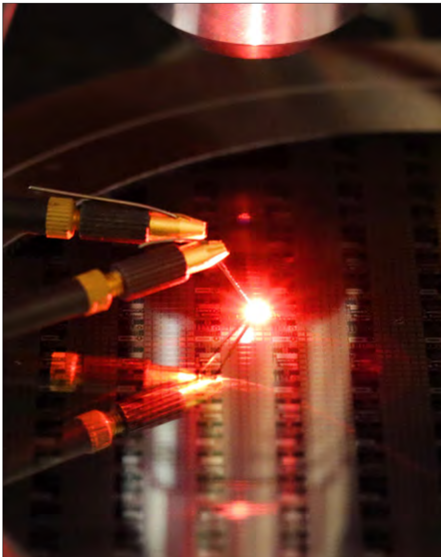
Well red: Plessey's GaN on Silicon-based Red LED.
