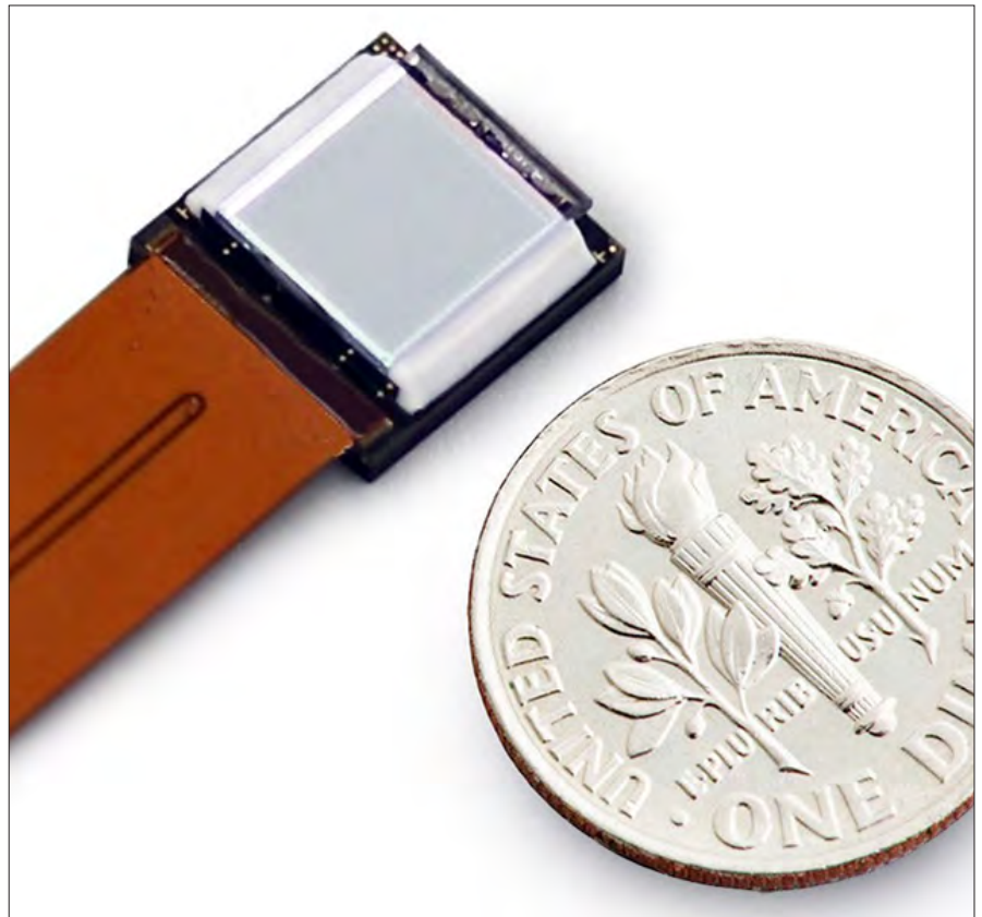
CP2K234 microdisplay based on Liquid Crystal on Silicon.
