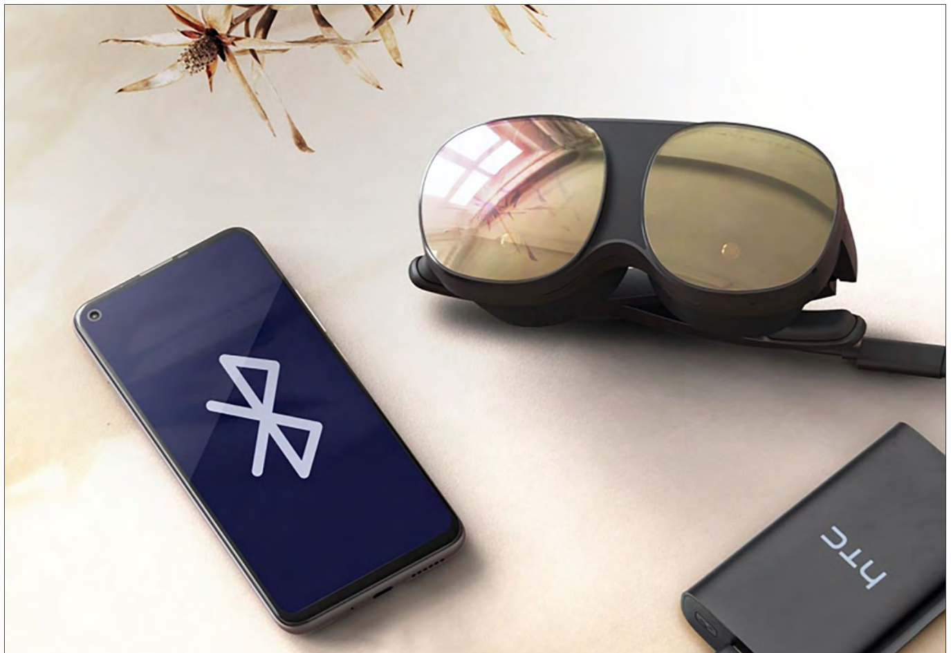
HTC's 'Vive Flow' eyeglasses for VR use so-called “pancake” lenses to reduce the size and weight of the design - and also feature binocular-like adjustable diopter lenses for personalized focusing.
