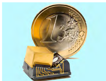
The basic element of future large-scale displays: A Trixel with a movable mirror.
