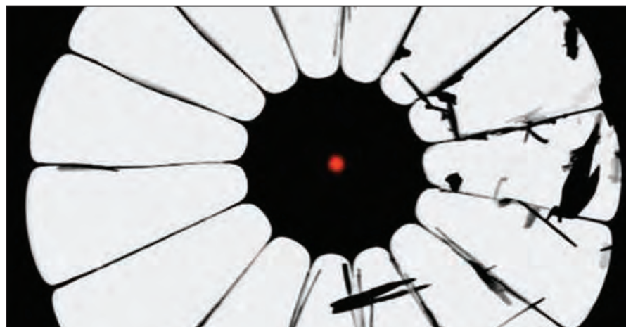
High-numerical-aperture photonic crystal fiber allows lensless focusing in a tiny endoscope - at an unparalleled resolution by complex wavefront shaping.
