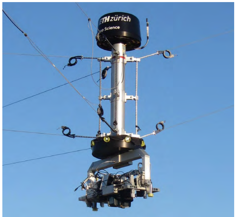
Sensor head of the FIP: RGB and NDVI DSLR camera, laser scanning device, thermal camera, spectrometers and operational camera can take data of the field automatically.
