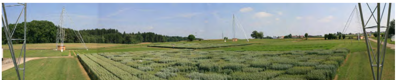
Overview of the FIP area of about 1 ha covered by the system. Three of the poles which carry deflector roles on top and the winch houses at their base are visible.
