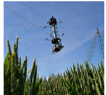
The sensor head only takes a few seconds to capture a wheat plot.
