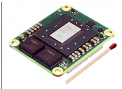
Smart chip: Tulipp's proposed reference platform hardware implementation.
