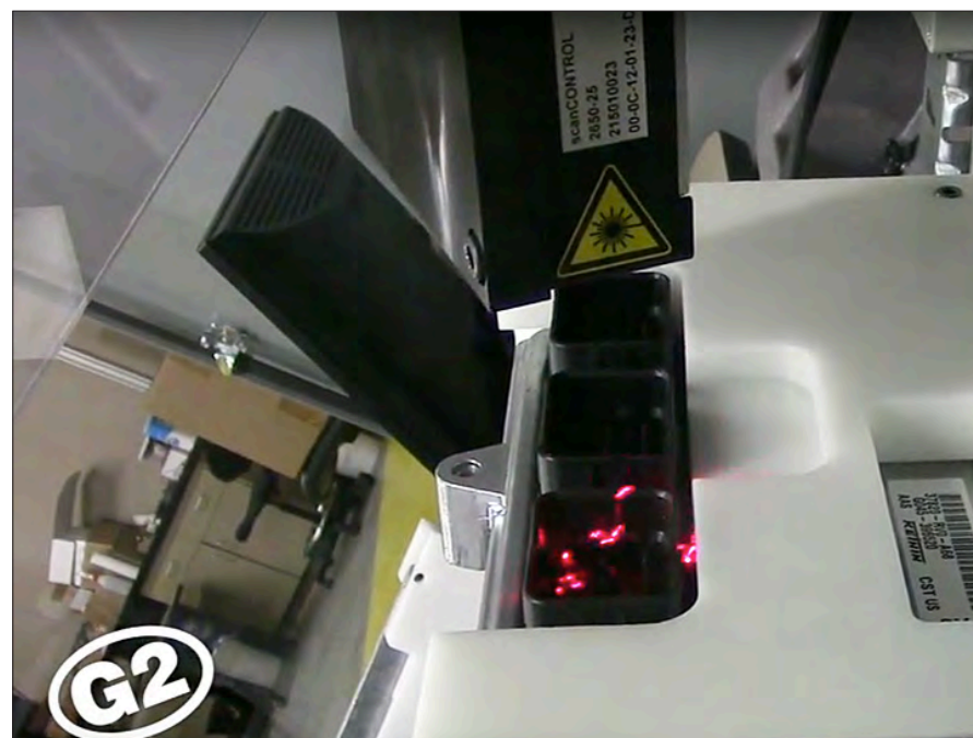
The 3D inspection system from G2 Technologies combines a machine-vision based, non-contact 3D inspection system, a cleaning station, and electrical test and engraving stations.
