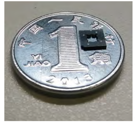
The MEMS component that provides hyperspectral imagery in Unispectral's smartphone-compatible technology. The Israeli startup recently closed a $7.5M round of series A venture funding.
