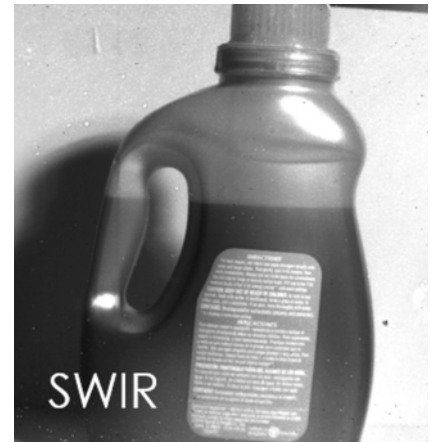
InfraRed image using SWIR Vision Systems Acuros™ Camera detects liquid fill levels for quality control on factory manufacturing lines.
