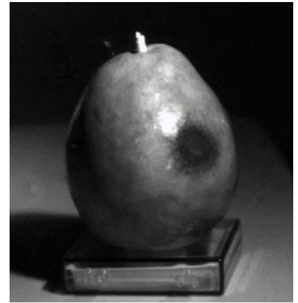
InfraRed image using SWIR Vision Systems Acuros™ Camera detects subsurface bruising valuable for food sorting applications.
