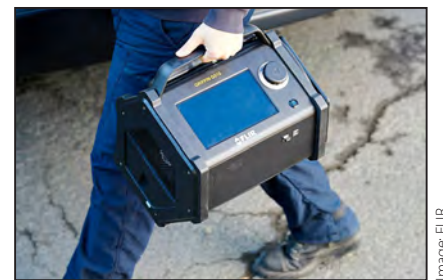
FLIR's Griffin G510 person-portable gas chromatograph mass spectrometer.
