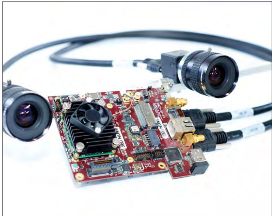
Stereo camera and the embedded system installed on the drone.
