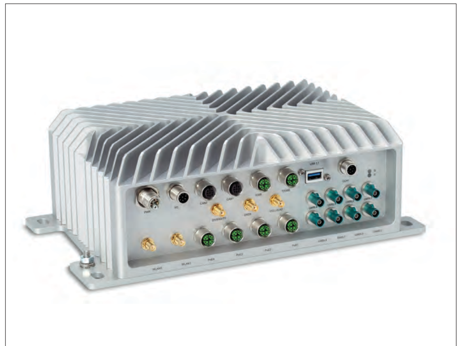
Syslogic's rugged AI embedded AR computer, the RPC RML A4AGX model.
