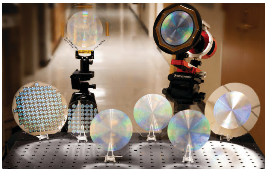
This 10-centimeter-diameter glass metalens can image the sun, the moon and distant nebulae with high resolution.
