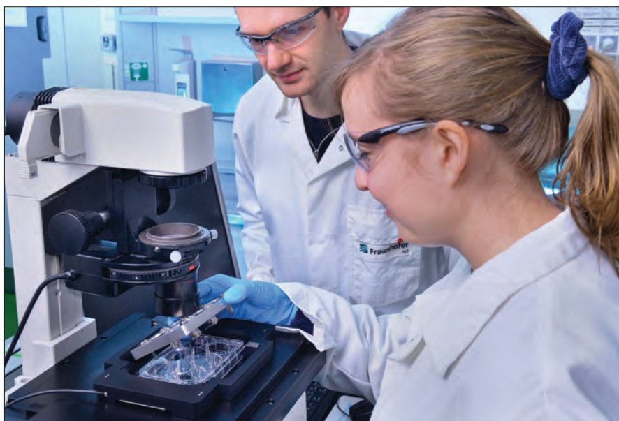
Researchers at Fraunhofer ILT are testing the LIFTOSCOPE for AI-assisted, fully automated high-throughput sorting of living cells by pulsed laser radiation.
